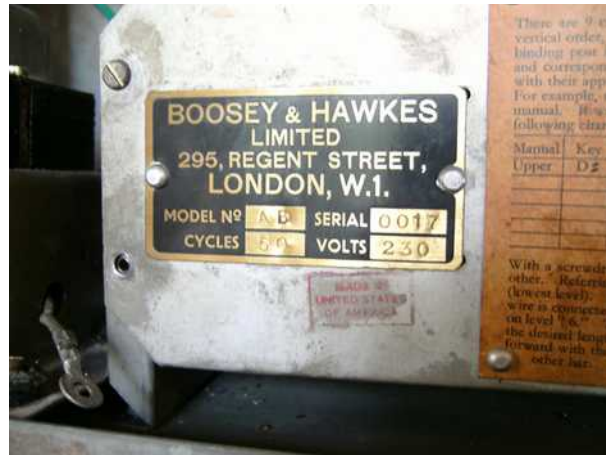
Model AB (above) showing two of the four original rivet holes from the Hammond serial plate underneath the Boosey & Hawkes serial plate
